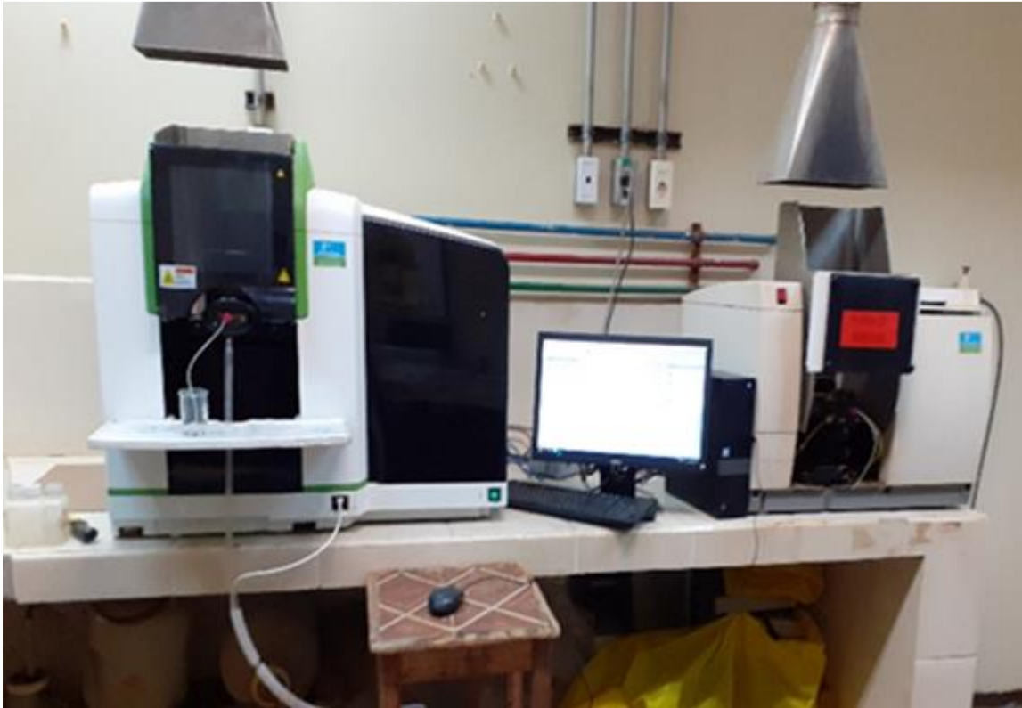
Figure 11.2: Atkin Absorption Systems, Perkin Elmer PinAAcle and AAnalyst 900
