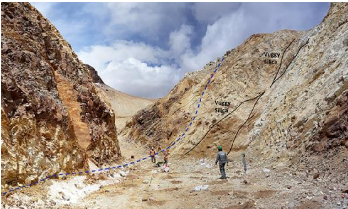
Figure 7.9: View to the Southeast of the Claudia Eugenia Pit showing vuggy silica with variable thicknesses in sigmoidal loops
